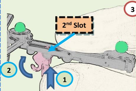
1. Guide the U-hook into the 2<sup>nd</sup> slot.
