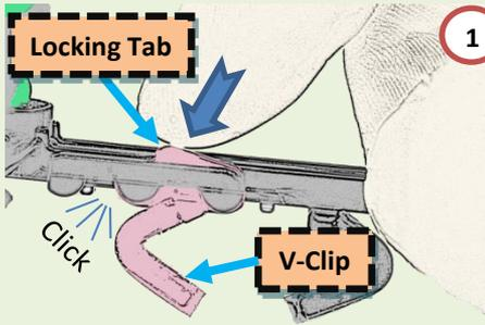
Unlock the V-Clip by pushing the Locking Tab with your finger. A click will be heard when the V-Clip is unlocked.
