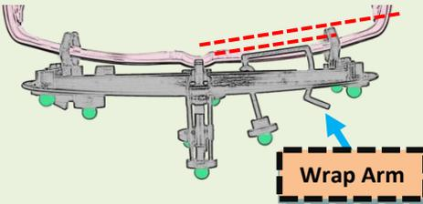
Move the wrap arm front and back until its back edge is parallel with the frame as viewed from above.
