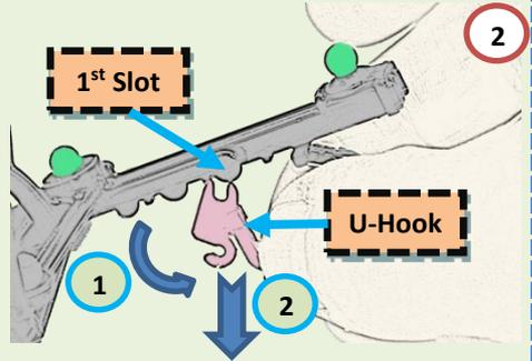
1. Rotate the V-Clip to its removal position.
