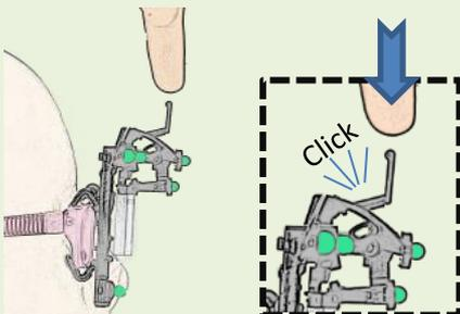
Unlock the brake arm on the EY-Stick and ask the patient to wear the frame. The customer is asked to sit or stand, depending on how the frame will be used.
