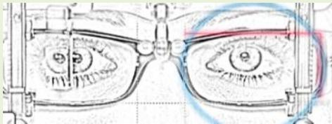
Line up the frame measurement lines with the top and right-most edge of the customer's left lens. Adjust the effective diameter slider until the circle is as small as possible but still encompasses the entire lens.
